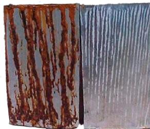
**Salt Spray Test:** Coated panels were exposed for 14 days to salt spray per ASTM- 117 test procedure at an independent testing lab. The results conclusively indicate that metal surfaces protected using Flexi-Film® provide superior resistance to environmental elements.
